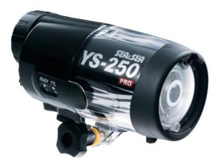
The YS-250PRO is designed for demanding professionals, packed with revolutionary new features to meet the challenges of digital photography. A large circular arc tube emits a powerful flash at guide number 32 (its value on land, ISO 100/m) when power is set to FULL. It provides incremental manual flash power adjustment in 12 steps for graduations of light.
