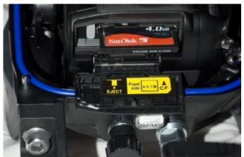
It is possible to change the card (loading sideways) while the camera is locked in the housing. 2 Pins prevent accidental misalignment of the back when closing the housing.
