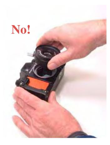
Never remove a lens like this as water droplets can fall into the throat of the camera and get onto the shutter blades
