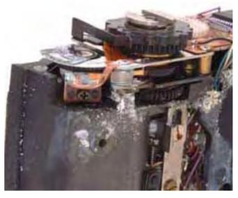
Corosion can clearly be seen around the frame counter assembly which also contains the main power contacts.
