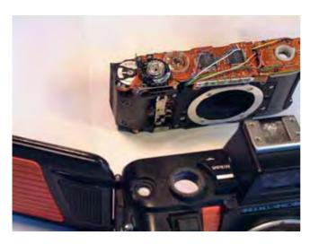
The inner body of a Nikonos V is a very snug fit in the main outer body. This keeps the camera small but any slight amount of water getting into the camera will cause problems with the electronics and mechanics
