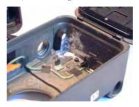
It is only when the inner body is removed that signs of corosion can be seen just under the frame counter window.
