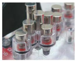
A balance has to be achieved to allow the user to push a spring loaded control yet not allow water pressure to do so as well. The solution is a combination of spring strength and O ring tension to achieve waterproof operational success.
