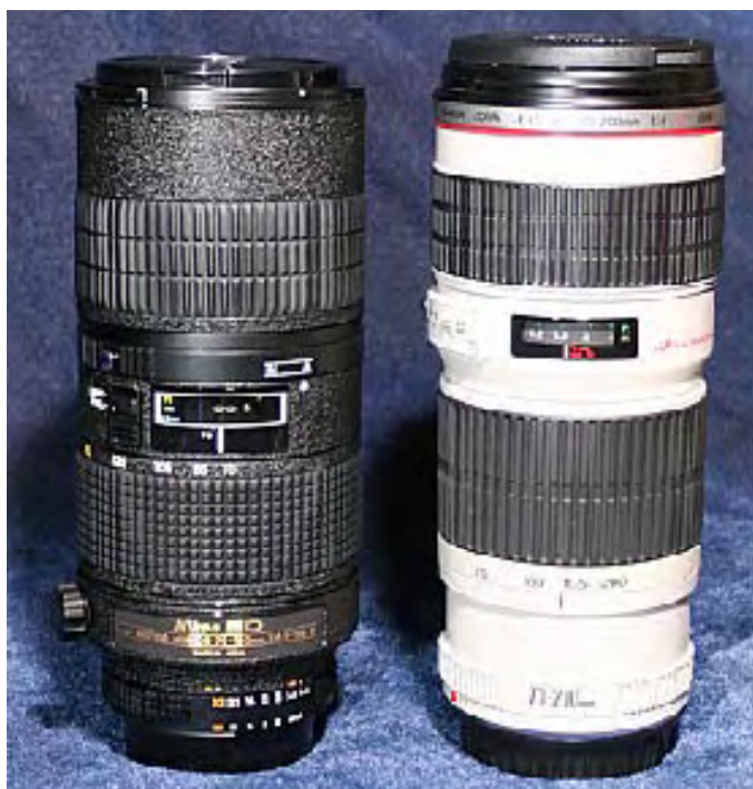
The Nikon 70-180 Micro and the Canon 70-200 F4L. The Canon lens has a removable tripod collar, which is not shown. The tripod collar on the Nikon lens is not user-removable.
