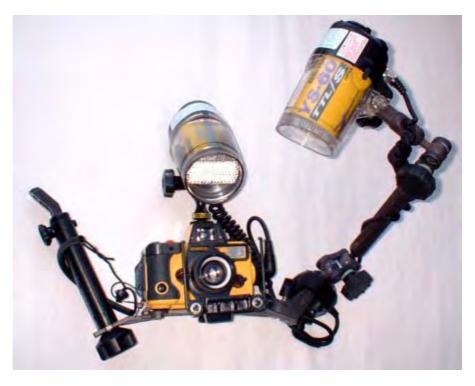
All of the macro images in this article were shot using the Sea & Sea MotorMarine II-EX with either a Macro Lens 2T (1:2) or 3T (1:3) conversion lens. Illumination was provided by dual Sea & Sea YS-60TTL S strobes synchronized with a 4 Pin Dual Sync Connect, mounted using Sea & Sea's Hot Shoe Arm and Sea Arm V. A Sea Arm IV was used as a handle for carrying the system.
